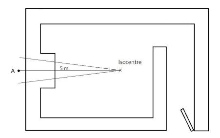
(a) The above diagram shows the structural layout of a treatment room installed with a 15 MV linear accelerator with maximum output dose rate of 400 MU/min. Please calculate the thickness of the concrete required in order to reduce the radiation dose rate at point A to the limit as stipulated in Regulation 17(1) of the Radiation (Control of Irradiating Apparatus) Regulations (Cap 303B).
